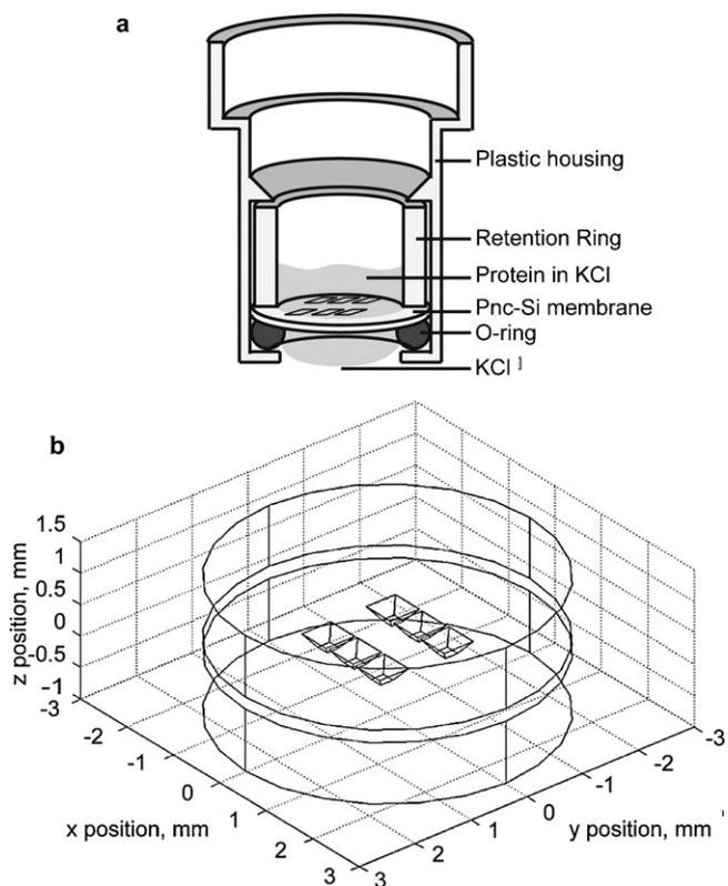
**Fig. 2.** Experimental setup and 3-D computational diffusion model. (a) Schematic of experimental setup. (b) CAD model of experimental system: 6 windows covered with 15 nm thick membrane material separate two fluid wells.
