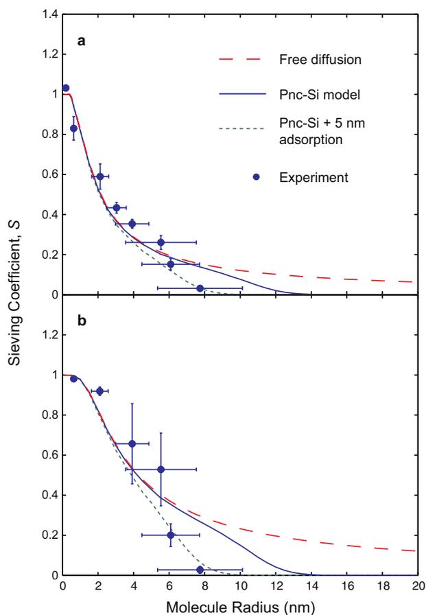
**Fig. 9.** Experimental and 3-D model sieving profiles for pnc-Si separations at (a) 24 h and (b) 48 h using DLS sizing for experimental data. The sieving profile (solid line) deviates from free diffusion (dashed line) near the physical pore size cutoff. The largest molecules deviate from the theoretical sieving profile. We plot an additional simulation with an added 5 nm protein adsorption ring to the pores, and this adjustment fits the data for both 24 and 48 h.
