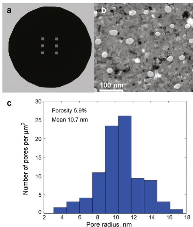
**Fig. 1.** Pnc-Si membrane. (a) 6.5 mm diameter silicon chip with six 0.2 mm  $\times$  0.2 mm freestanding pnc-Si membranes. (b) TEM micrograph of nanometer scale pores in 15 nm thick pnc-Si membrane film. Pores are white ellipsoids and nanocrystals are black spots. (c) Pore characteristics as determined from image processing of 2  $\mu\text{m}$  squared area of micrograph.
