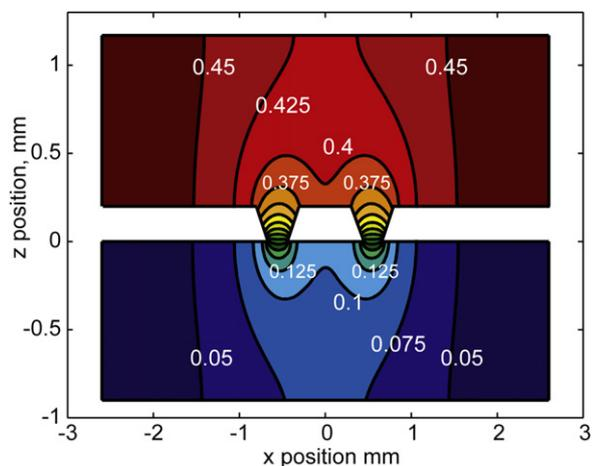
**Fig. 8.** Slice through 3-D model after 10 h of diffusion of a 5 nm radius molecule. Concentration isolines show diffusion through the membrane (at  $z$  position 0) from the retentate (top) to the dialysate (bottom).
